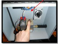
**5**. Push the control knob all the way in and hold. Immediately push the electric igniter button. Continue to hold the control knob while visually checking to see that the pilot light has lit inside the heating chamber along the burner.
