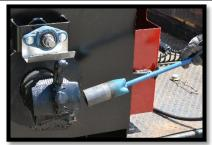
10. Once material has reached specified temperature, begin application. Heat may be required to allow material to flow from the valve during the first dispense using the supplied torch. Do not apply heat to the bearing, may cause premature failure. Add more material as required using the same method as steps 6 and 7.
